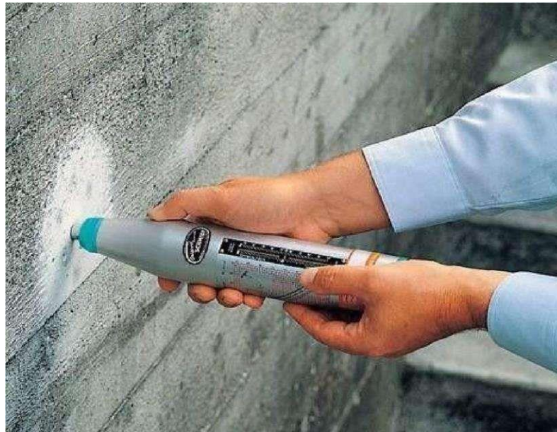
NDT test on concrete
